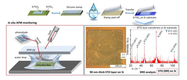
Transfert of the épitaxial film of SrTiO3 onto Si using
