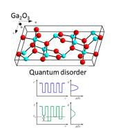
A new study shows that, through phosphorus doping of -GaO, an exceptional p-type conductivity is obtained at room temperature, as well as a metal-insulator transition. These results open avenues for improving power electronics, essential to power grids and transport systems, and contributes to wider adoption of renewable energies.
