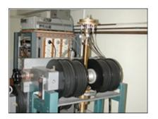
The second "high impedance-high temperature" (1e+10 Ohm) set-up is equipped with a 1.6 T electro-magnet in 80 K - 880 K temperature range.
